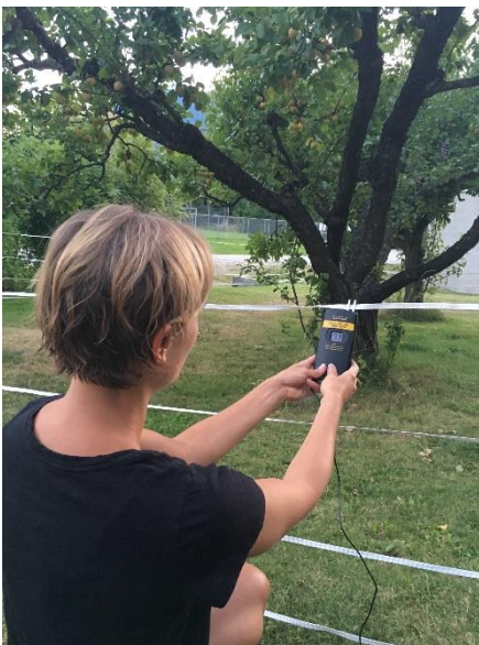
Figure 2: Testing the voltage of a temporary electric fence
