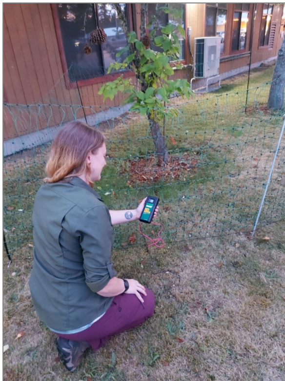
Figure 6. The WCC testing the voltage of the demonstration electric fence at the Nakusp electric fence workshop. Photo credit: Gillian Sanders.
