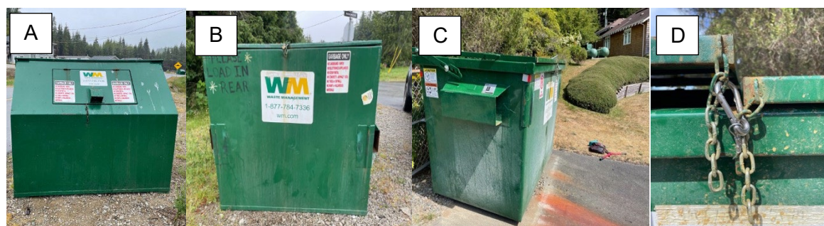
Figure 8. A & B) Photo of front and backside of non-bear-resistant bin model without bear-resistant bars in Bamfield and Anacla. C) Photo of side view and front view of non-bear-resistant bin model without bear-resistant bars in Bamfield and Anacla. D) Photo of failed carabiner/chain securing mechanism due to damage.
