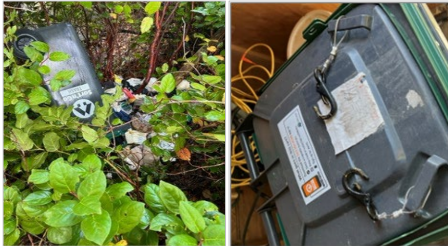
Figure 6. Bears most often dragged unanchored poly carts into secluded locations and eventually learned how to break carabiners.
